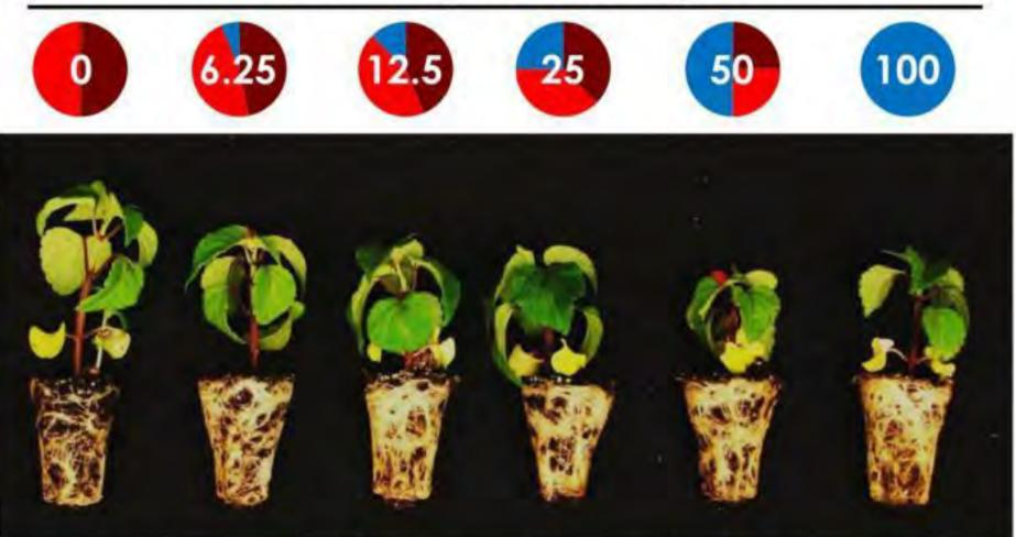
B=blue LED peak=446 nm; R=red LEDs peaks=634 and 664 nm
